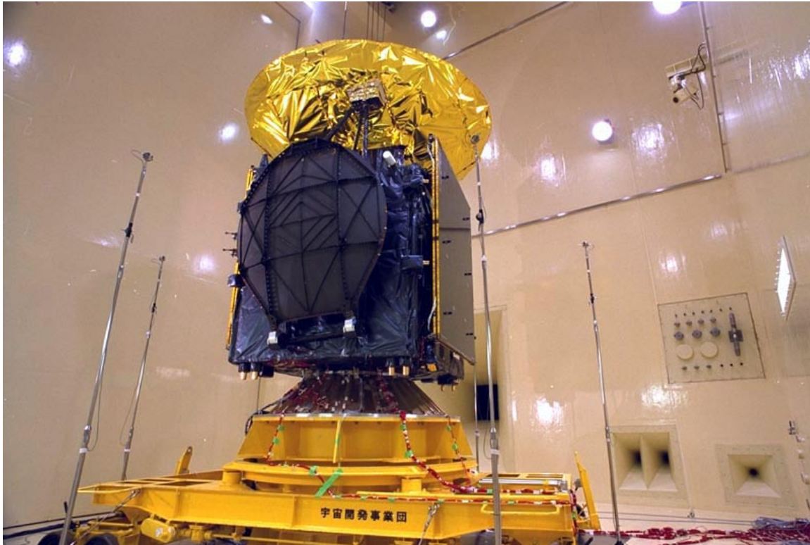
Figure 1-1. Data Relay Test Satellite inside Acoustic Chamber at Tsukuba Space Center, Japan
