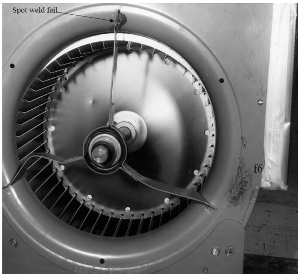
Figure 4. Blower Failure with Bent Spider Members
