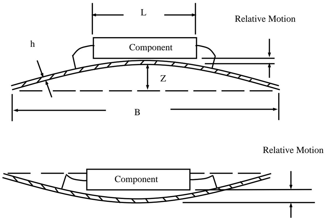
Figure 3. Circuit Board Bending Deflection
